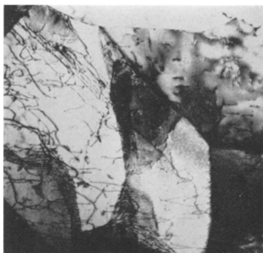
Figure 2 Electron micrograph of substructure in the forged ingot ( \times 27\,500 ).
